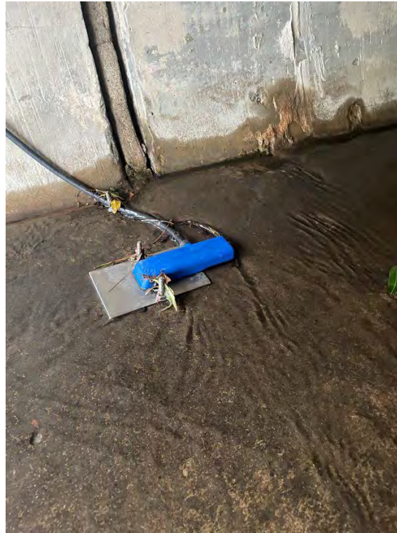
Figure 4-6. Example of Flow Sensor Installation
