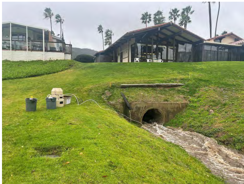
Figure 4-8a. Example of Temporary Automated Sampler Setup
