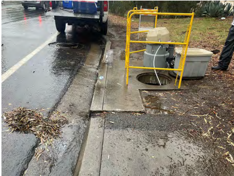
Figure 4-8b. Example of Temporary Automated Sampler Setup
