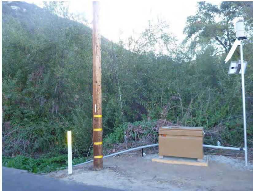
Figure 4-7. Example of Permanent Automated Sampler Enclosure
