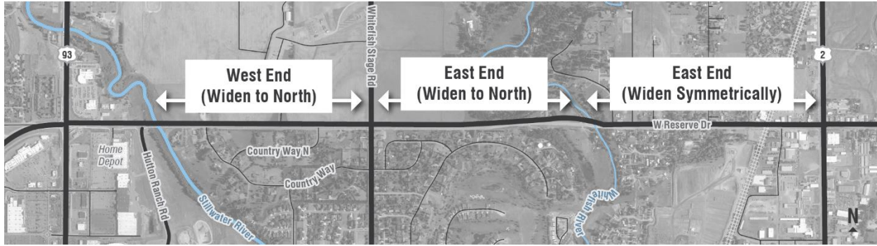
Figure 11: Corridor Widening by Segment
