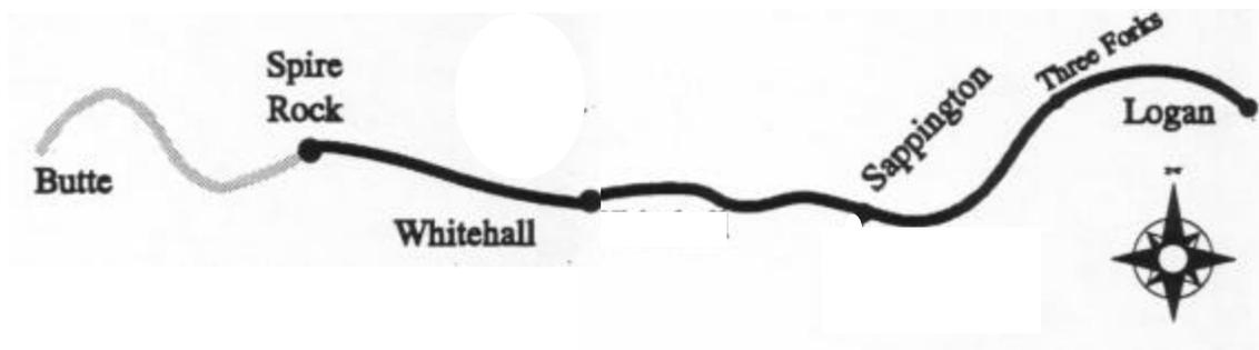
The Logan-Spire Rock (a railroad location 11.8 miles west of Whitehall) Branch Line is 50.7 miles in length and has a maximum speed of 40 mph (FRA Class 3). Train control is by TWC.<sup>73</sup> Maximum car weight is 143 tons. Weight of rail on this line is a combination of 100, 110, 112, 115, 131 and 132 pound; except for a few segments of CWR, this is bolted rail.
