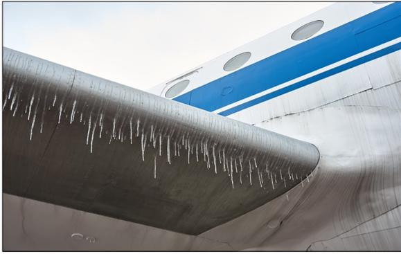
Aircraft ice is bad news for most small general aviation aircraft. It destroys the smooth flow of air over the aircraft which in turn increases drag and decreases lift. Structural aircraft ice comes in a few different forms.
