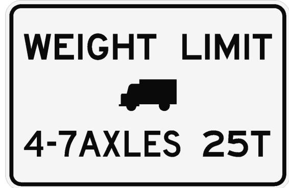
The new posting on the MT 200/US 87 Drainage Bridge applies to SHVs; it limits the maximum gross vehicle weight of single-unit vehicles with 4, 5, 6, or 7 axles to 25 tons.
