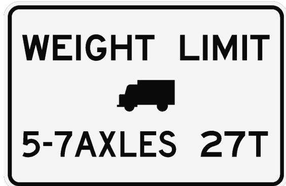
The new posting on the Butte Creek Bridge applies to SHVs; it limits the maximum gross vehicle weight of single-unit vehicles with 5, 6, or 7 axles to 27 tons.
