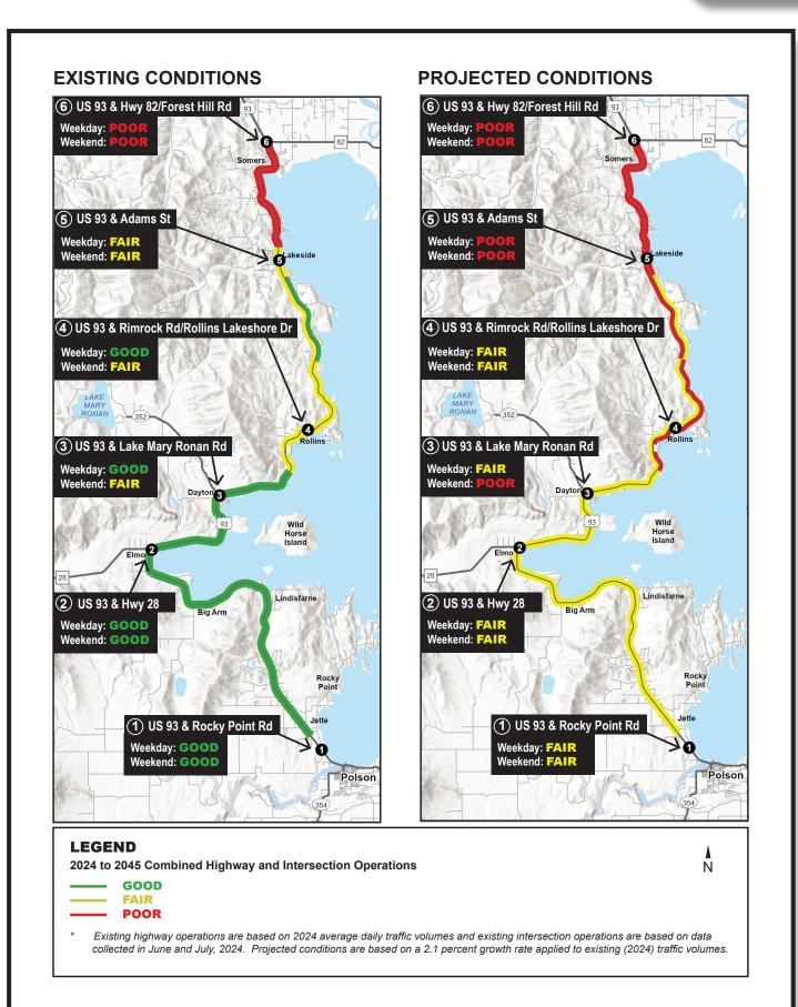
**Figure 8: Existing and Projected Traffic Conditions**
