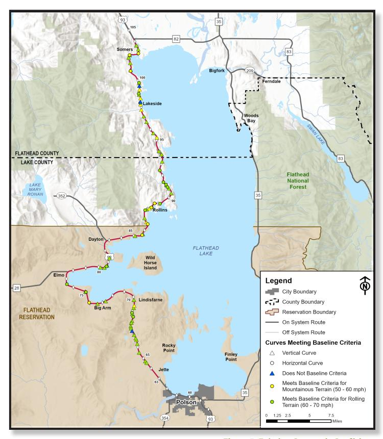
**Figure 5: Existing Geometric Conditions**
